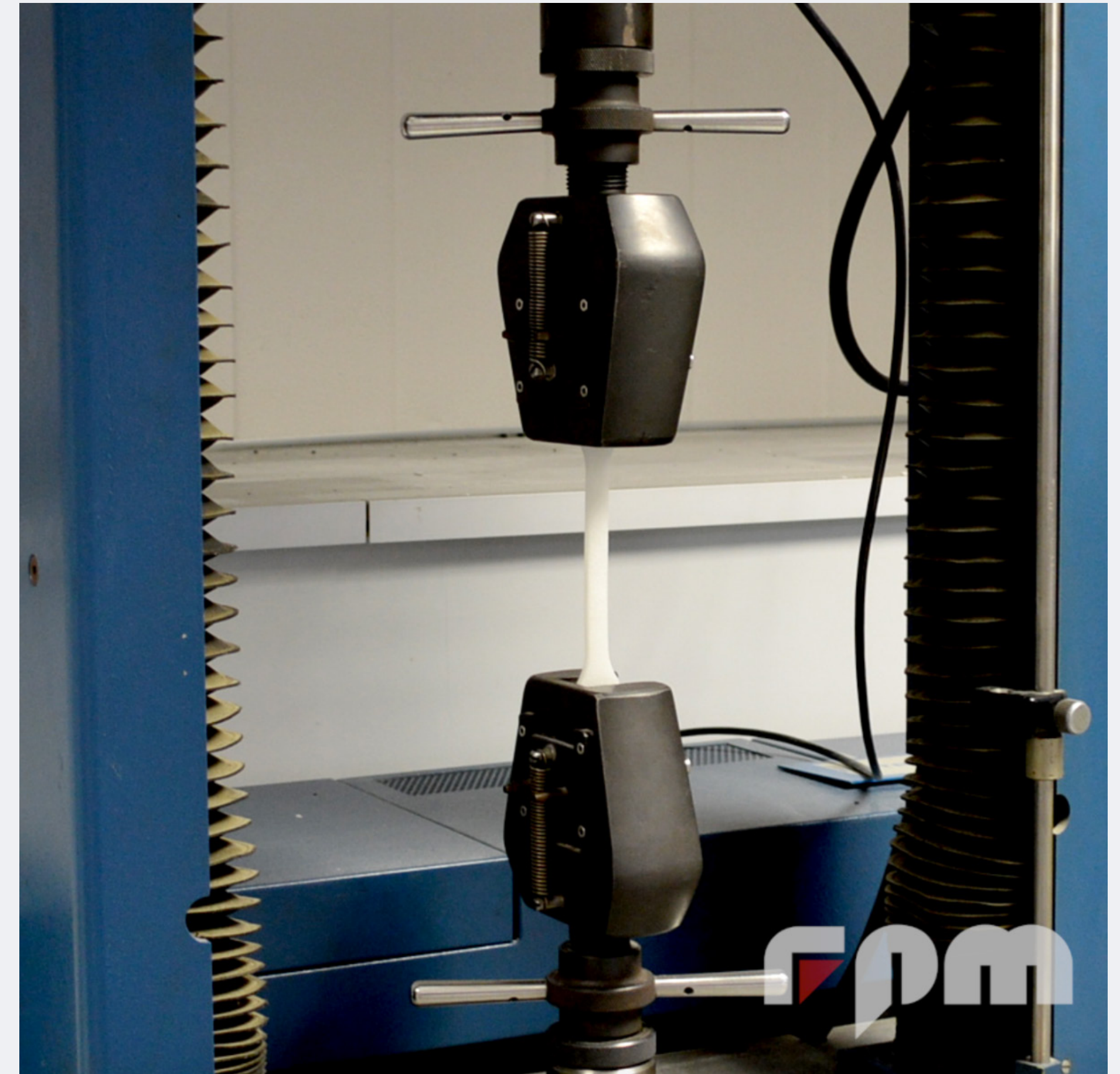
Tensile strength testing of EPU 41 at specific thicknesses to inform product design Image: rpm rapid product manufacturing GmbH
