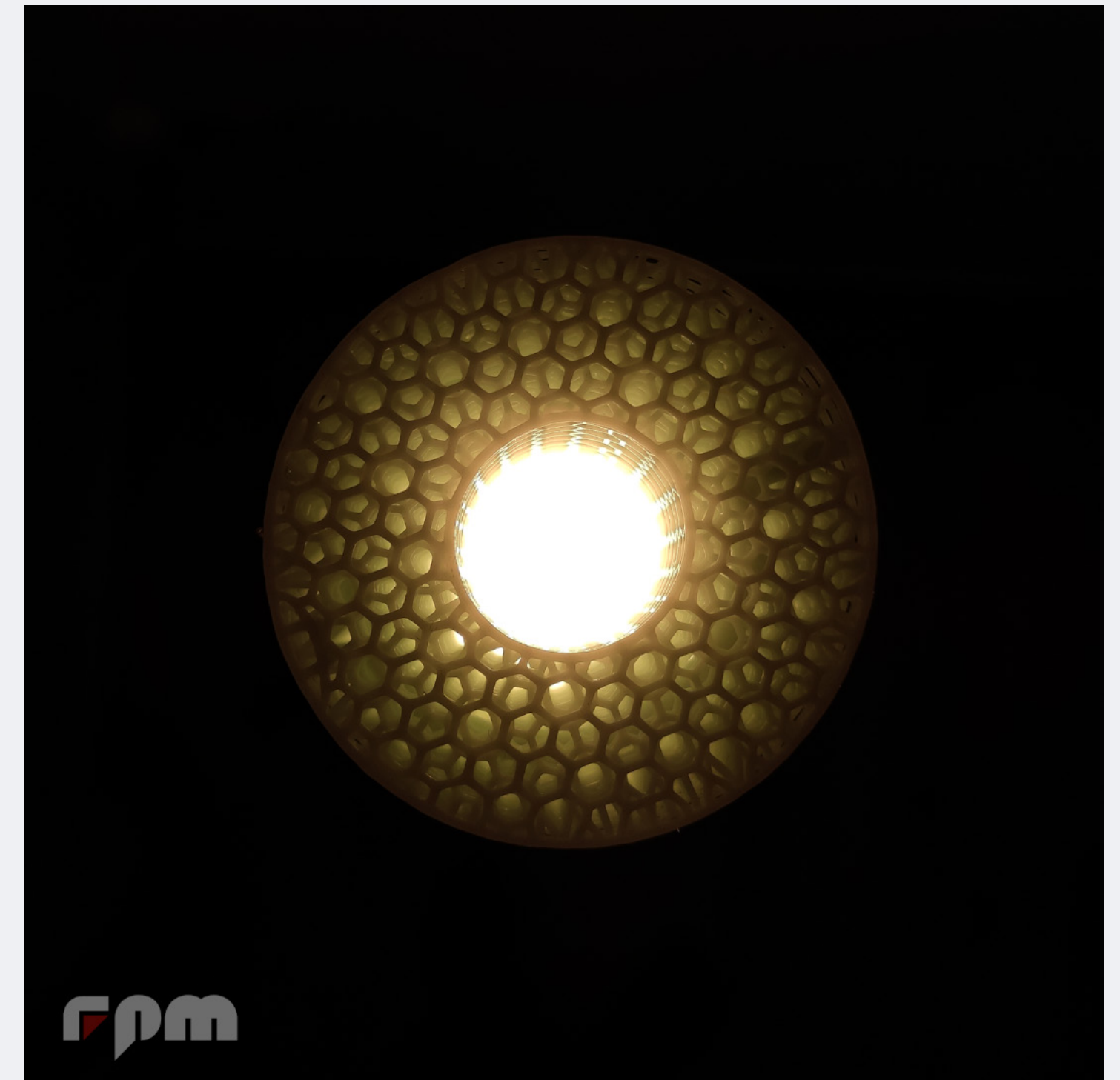
Circular lattice with inner channeling for testing mechanical properties produced as part of the German ZIM research grant (Central Innovation Program for German SMEs) Image: rpm rapid product manufacturing GmbH
